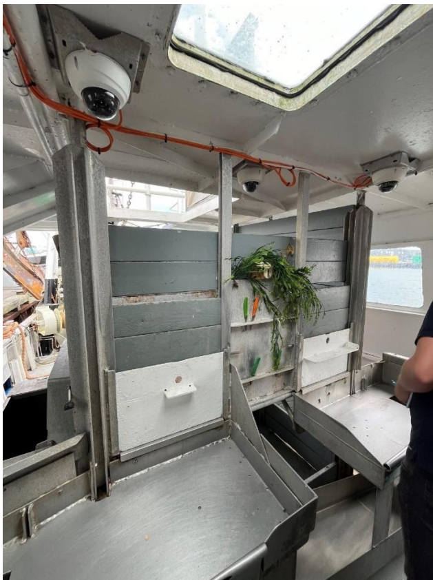
Figure 5. Sample images illustrating the diversity in layouts for fishing vessels equipped with sorting tables, where camera angles and catch sorting areas pose significant challenges for automated catch documentation.
