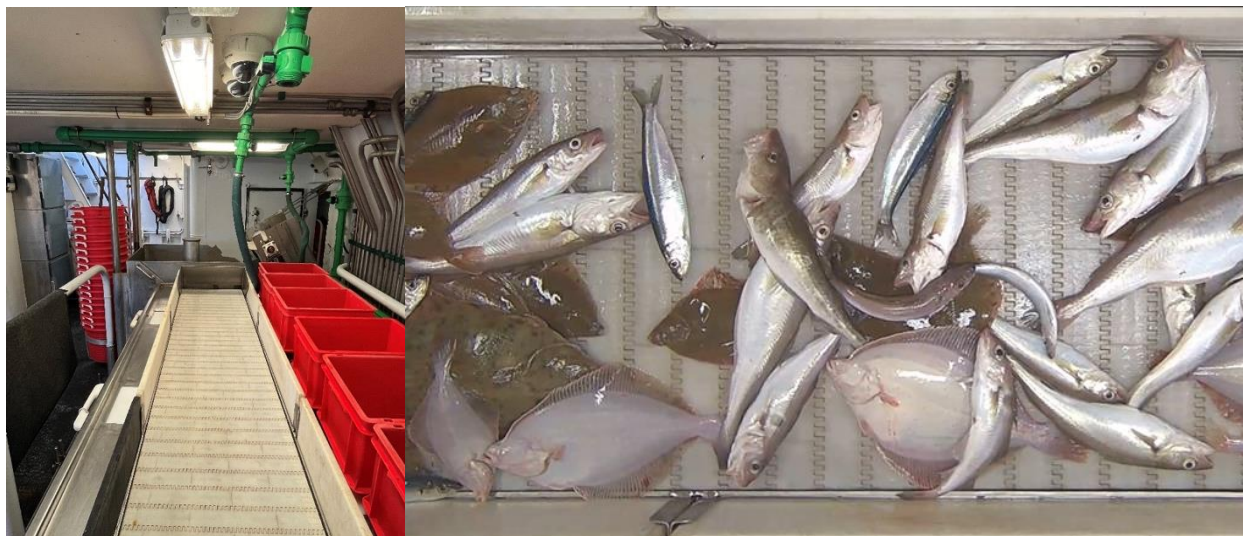
Figure 4: Sample images from fishing vessels equipped with conveyor belts illustrating the differences in layout and the associated image acquisition scenes from the EM cameras placed above the conveyor belts.
