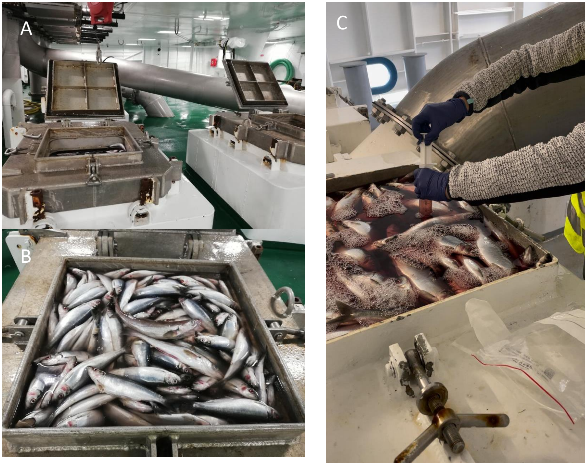
Figure 3. Examples of storage tanks used for holding the catch on an industrial pelagic fishing vessel, where water samples for environmental DNA (eDNA) analysis are collected to estimate catch composition. Each tank can hold tens to hundreds of tons of fish, typically containing approximately 70% fish and 30% water, with proportions varying by target species and season. To maintain the catch in optimal condition, refrigerated seawater at -1.7^{\circ}\text{C} is recirculated and the tanks are often interconnected. (B) Surface view of a tank showing Atlantic herring ( Clupea harengus ) alongside a bycatch species, whiting ( Merlangius merlangus ). (C) Collection of water samples for eDNA analysis performed at landing facilities using a sterile syringe.
