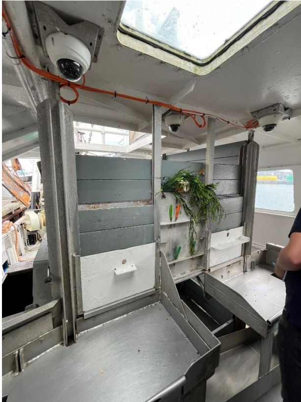
Figure 3. An example of an image acquisition scene from an electronic monitoring camera placed over a sorting table.
